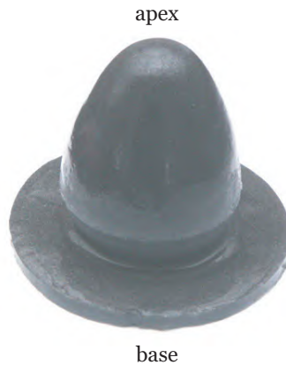
Figure 5-5: Phantom of the left ventricle, made from a polyvinylalcohol (PVA) solution mixed with 1% graphite powder.
