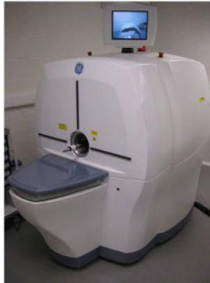
Figure 3.7: The setup of the \mu CT scanner (reproduced from [7]).
