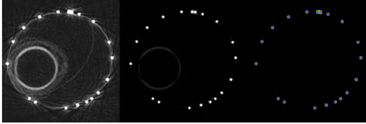
FIGURE 2.3: \mu CT slice of a scanned stent graft. Full ranged window view (left), altered window level and reduced width (middle), rainbow color lookup table, showing a good threshold for wire separation.
