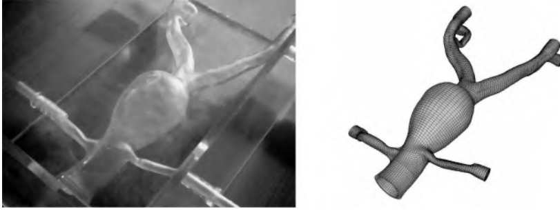
FIGURE 5.2: Silicone model (l.) and discretized FEA model (r.).
