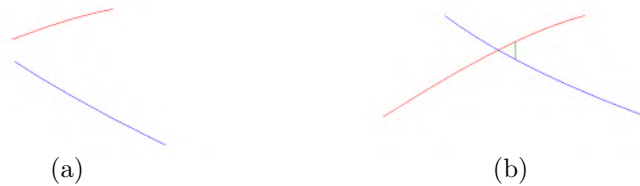
Figure 4.7: Creation of unit cell of crossing and connected struts (b) from a rescaled and mirrored, skewed (a) bumped strut.
