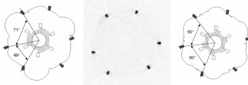
Figure 3.15: Cross section at the end of the transient stent expansion, showing that a trifolded balloon causes a non-uniform strut distribution (left panel: simulation; center panel: experiment), whereas a sixfolded balloon (right panel: simulation) results in a homogeneous strut placement.
