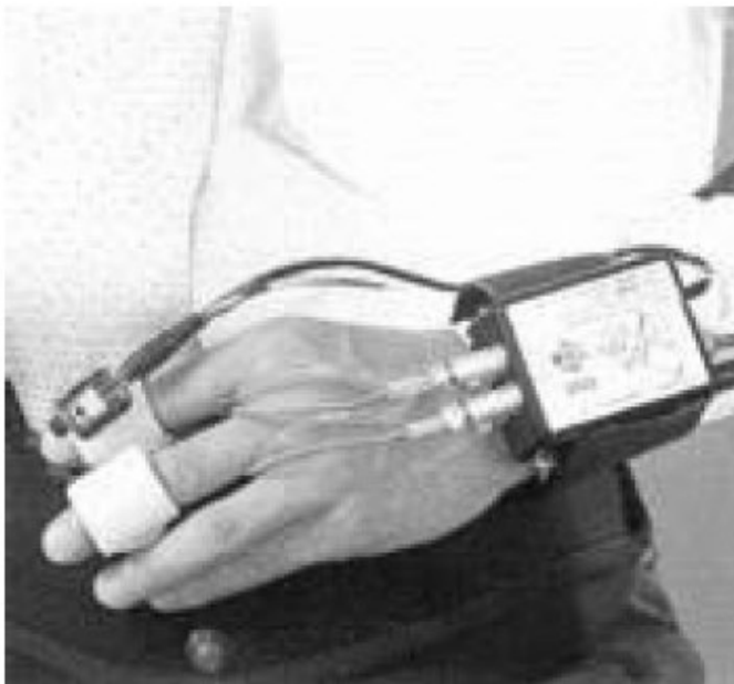
Figure 4.5 : Measuring finger arterial waveforms with the Penaz method (Finapres device, FMS Finapres Medical Systems, Arnhem, NL).
