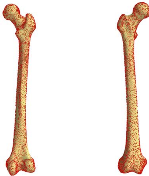
Figure 5.29: Posterior and anterior views of the final result of the fitting of the aligned data point cloud (in red) and the reference mesh.
