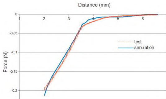
FIGURE 7.3: Flat plate test results and numerical approximation.
