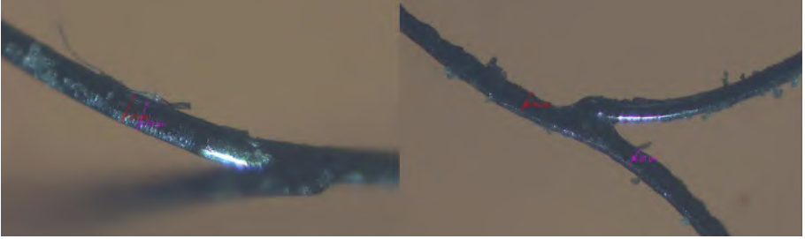
FIGURE 7.1: Optical Microscopy measurements of the Enterprise stent. A detail of the stent struts shows the measurements of the thickness (left) and width (right). Irregularities of the surface are imputable to dirtiness of the sample.
