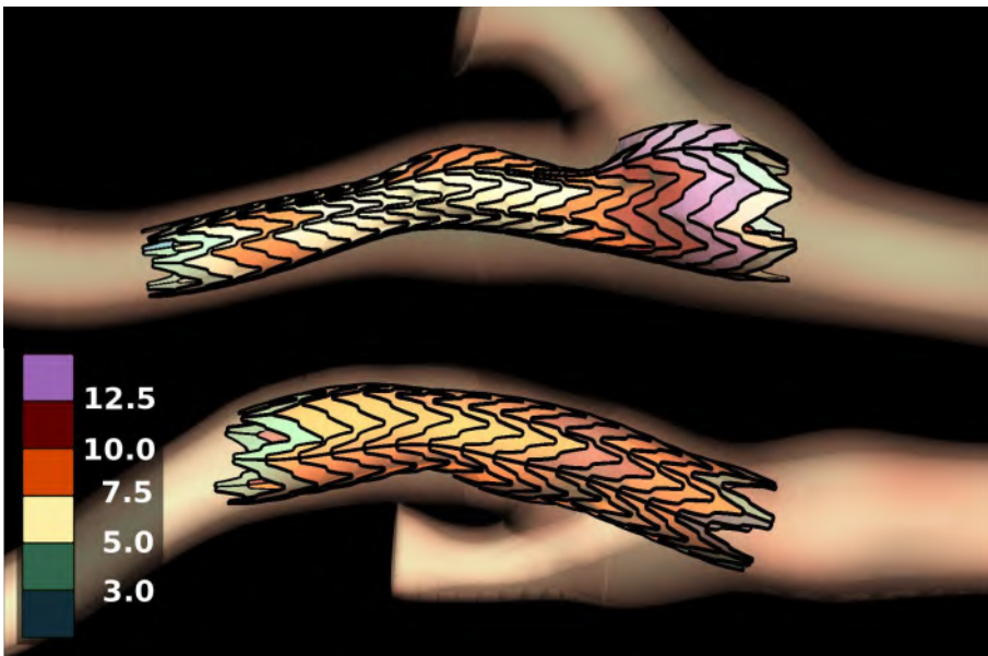
FIGURE 5.8: Free cell areas (FCAs) of the implanted stents (in mm^2 ). Top: patient A, bottom: patient B.
