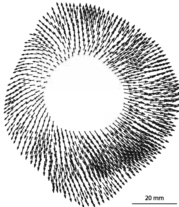
Figure 6.1: Interpolation of TMRI registered diastolic tissue displacement from the LV top basal short axis image slice to top surface nodal displacements of the finite element mesh.
