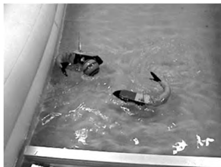
Figure 2.9: Carangiform fish robots swimming in an aquarium, developed by Yu et al. [41].
