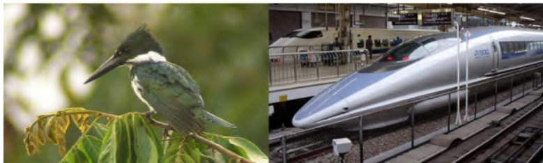
Figure 2.7: The shape of the kingfisher's head was used to design the nosecone of Japanese bullet trains [35].
