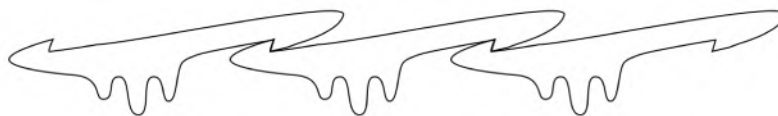
Figure 6.8: Conceptual drawing of a bio-inspired structure with high bending flexibility and high radial stiffness. The design has radial symmetry.
