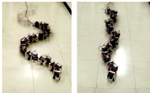
Figure 2.14: Snake-like robot developed by Wu and Ma [56] at different undulation wavelengths and amplitudes.
