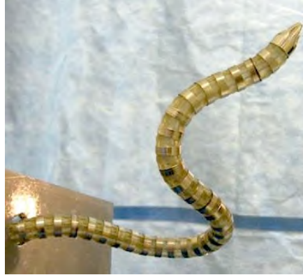
Figure 2.18: Bio-inspired robot designed to assist in minimally invasive cardiac surgery [65].
