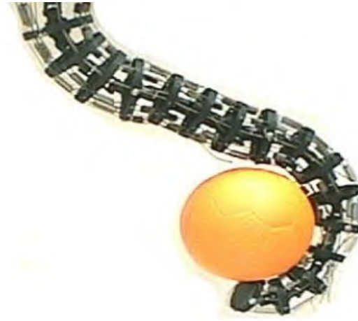
Figure 2.16: Manipulator inspired by the elephant trunk [63].
