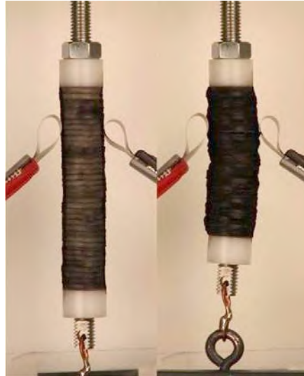
Figure 6.6: Muscle-mimicking actuator made from electro-active polymers [127].
