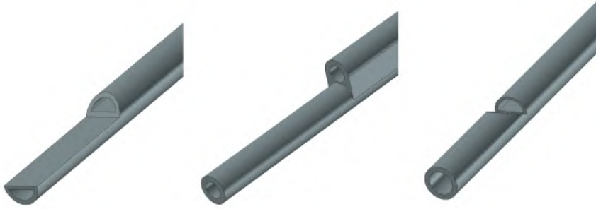
Figure 5.4: Examples of shotgun tip designs: (A) double-D as in Mahurkar catheter (Covidien, Dublin, Ireland); (B) oval-shape as in Quinton catheter (Covidien, Dublin, Ireland) and (C) round tip with double-D lumen as in the DuraFlow and DuraMax catheter (AngioDynamics, Latham, NY, US).
