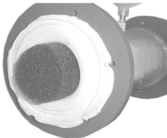
Fig. II-4: Top: overview of the lumped afterload. A: windkessel. B: resistor. C: valve. D: venous reservoir. Bottom: detailed view on the composition of the resistor, with the foam on the inside and the flanges of the membrane and the housing around it.
