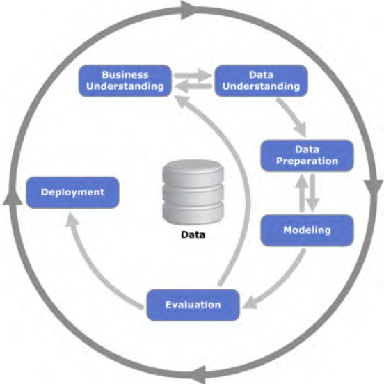
Figure 7.10: CRoss-Industry Standard Process for Data Mining model (CRISP-DM) by Shearer, Journal of Data Warehousing , 2000 [286]
