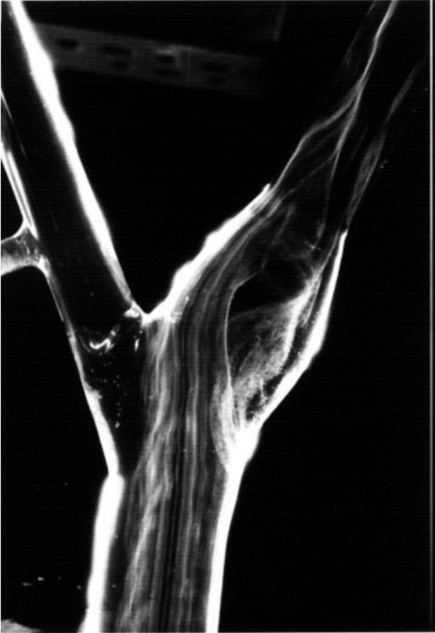
Figure 2.6: The flow separation region at the posterior wall of the internal carotid sinus is also the site of reverse velocities and secondary vortex patterns. Hydrogen bubble visualization of a carotid arteries model, adapted from [69].
