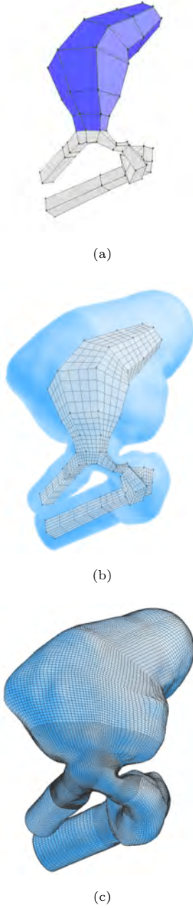
Figure 3.5: The mapping approach: (a) Multi-block structure, (b) block structured hex-core inside the geometry and (c) block structured hexahedral grid.
