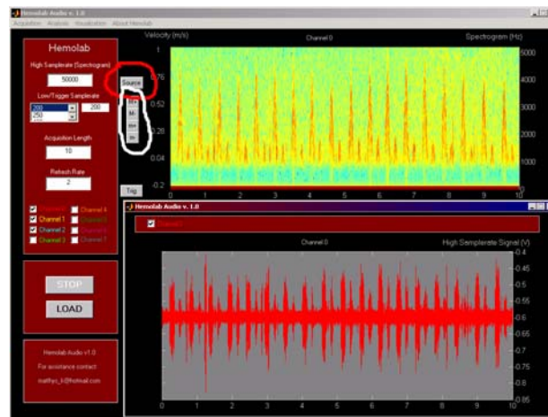
Figure 4–3 The new pop-up chart containing the high sample rate signal is enabled by pressing a toggle button (red circle) to the left of its spectrogram. Four push buttons (white circle) allow adjusting the scale to the left of the charts.
