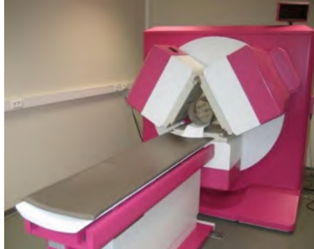
Figure 2.1: An Inter Medical Prism 3000 SPECT scanner. The three gamma cameras rotate around the patient and projections are obtained at a multitude of angles.
