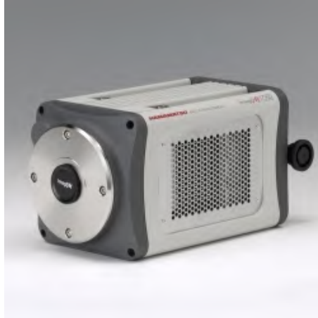
Figure 2.45: The Hamamatsu ImagEM EM-CCD camera uses a 512 \times 512 EMCCD sensor and has a frame rate of 70 frames/s. The sensor is cooled to -65^\circ C. Image courtesy of System Division, Hamamatsu Photonics K.K.
