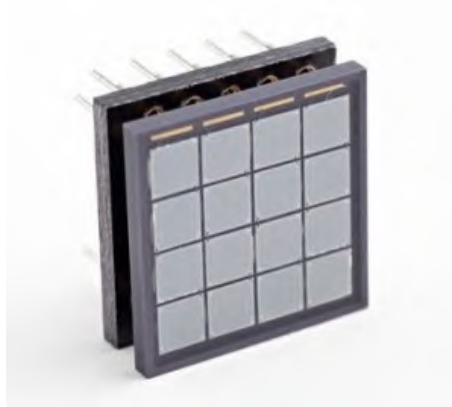
Figure 2.42: A SensL SiPM array; the pixel size is 3 mm \times 3mm (image courtesy of SensL).
