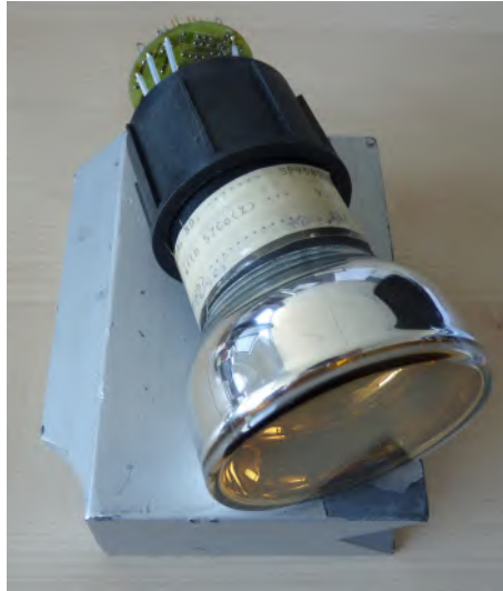
Figure 2.35: A Hamamatsu PMT that was once operational in a large clinical SPECT gamma camera. Its round package has a diameter of 7.5 cm.
