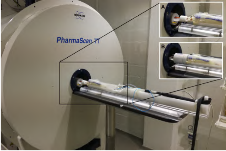
Figure 3.6: A small animal 7 T MRI system set up. The blue wire is part of the pressure pad that will send the respiration signal to the respiration monitor whereas the thick black cord contains tubes that deliver warm water to the warming blanket (blue pad on top of rat). The white nose cone delivers the anaesthesia (A). In this dissertation a quadrature volume coil was used to perform diffusion scanning and slides over the head of the rat (B).
