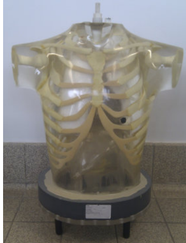
Figure 4.18: the Alderson torso phantom.
