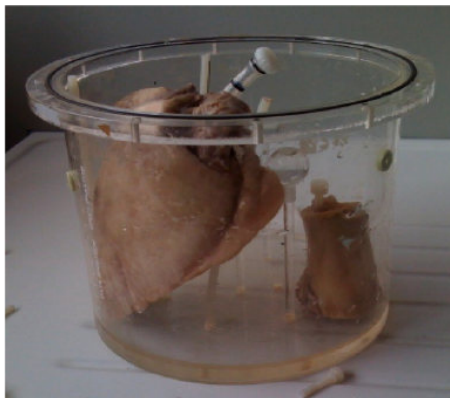
Figure 4.22: A thorax phantom contains one lobe of a pig lung and a bovine bone.
