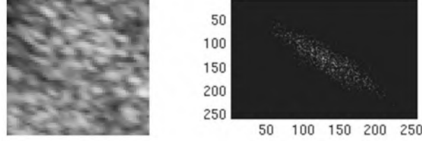
Figure 3.15: Left: a pathological flaring ROI. Right: a visualization of the corresponding co-occurrence matrix for d = 1 and \theta = 0 degrees. The whiter the entries in the matrix are, the higher their value is.
