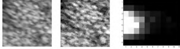
Figure 3.16: Left: the pathological flaring ROI. Middle: reduction of the ROI to 8 grey values. Right: Run Length matrix for d = 0 and \theta = 0 . The whiter the color, the higher the value of the matrix entry.
