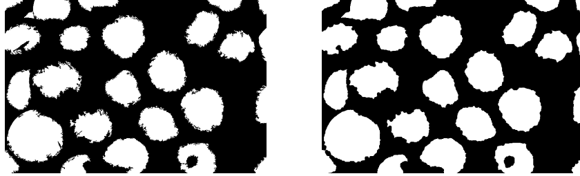
Figure 4.6: Left: original binary image. Right: closing by a square structuring element of size 5 \times 5 .
