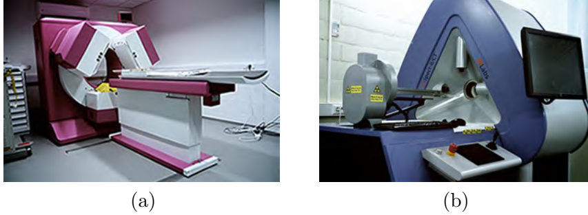
Figure 1.6: Examples of SPECT imaging scanners. (a) The Triple Head human SPECT scanner Prism 3000 NewTec, from Inter Medical; it supports both parallel-hole and fanbeam collimators. (b) The stationary small animal SPECT/CT system U-SPECT II, from MILabs, which uses multi-pinhole collimation. [Images obtained from [7]]
