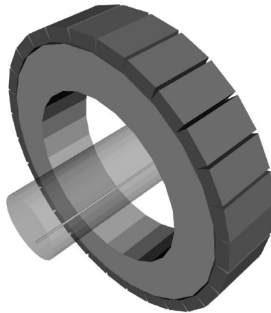
Figure 4.12: Simulation setup: GATE model of the Philips Allegro.
