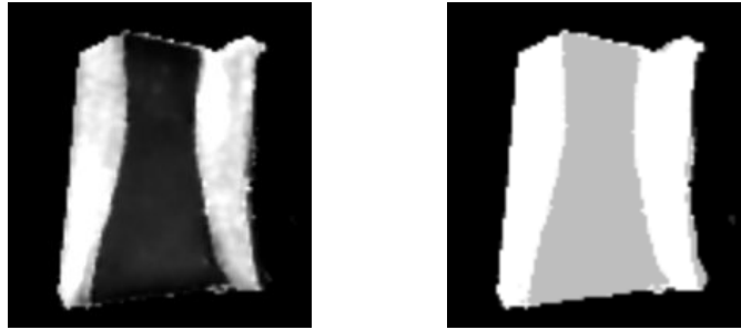
Figure 4.15: Slice through the corrected R_2 -map (left) and attenuation map derived from the corrected R_2 -map (right) of the bovine femur bone.
