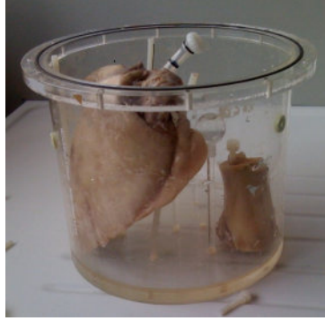
Figure 5.8: The assembled thorax phantom, containing a segment of bovine cortical bone and a lobe of pig lung.
