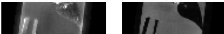
Figure 5.10: A sagittal slice of the FID (left) and gradient echo (right) image of the thorax phantom.
