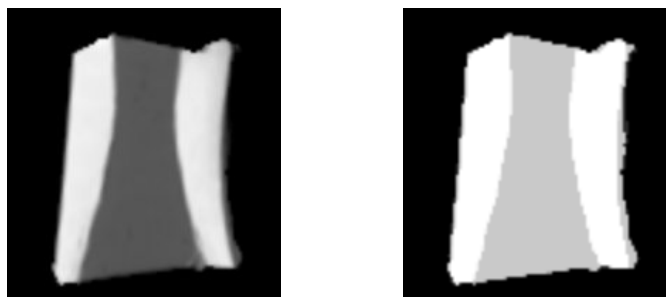
Figure 4.11: Slice through the CT (left) and segmented CT based attenuation map (right) of the bovine femur bone.
