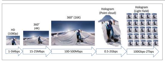
Figure 1. Bandwidth requirement evolution of video streaming services.
