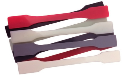
Fig. 2.16 Examples of tensile bars and large surface test moulding
