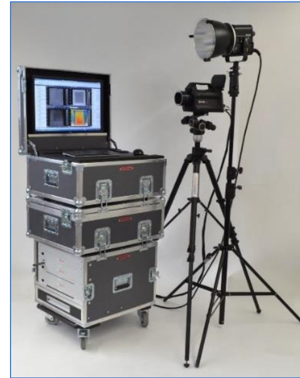
IR THERMOGRAPHIC SYSTEM
