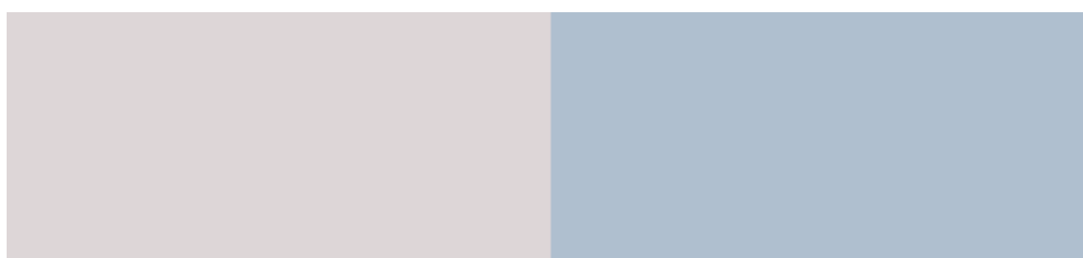
Fig. 32 Photocolouration of non-stabilised spirooxazine at first activation \Delta E = 16.56
