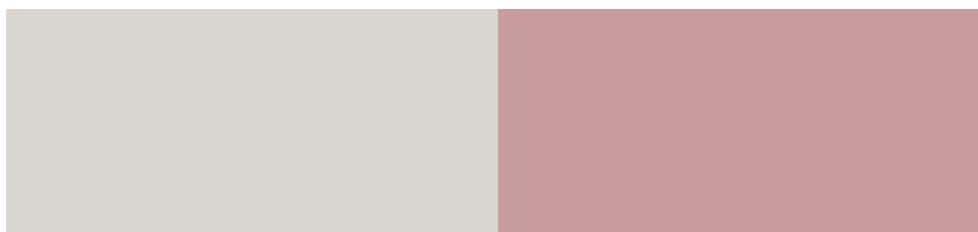
Fig. 30 Photocolouration of non-stabilised Ruby Red at first activation \Delta E = 21.03
