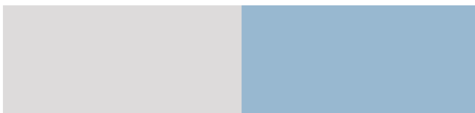
Fig. 31 Photocolouration of non-stabilised Oxford Blue at first activation \Delta E = 20.87
