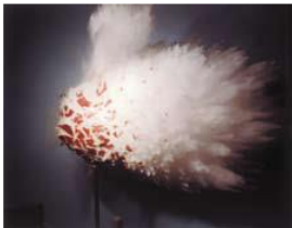
Demonstration of boundary effect on the temporary cavitation due to a high-energy rifle bullet: the apple literally explodes after the passage of the bullet.
