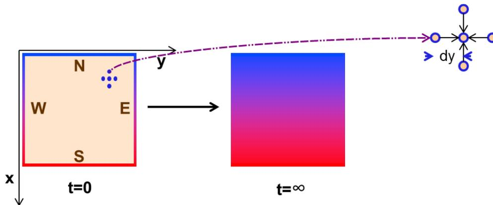
At the edges of the square, it is clamped to heat sources that keep the temperature constant at 0 on the north edge, at some fixed value  $\Phi > 0$  at the south edge, and a linear interpolation between 0 and  $T$  on the east and west edges, at all times. At time 0, the inside of the square is assumed to have the temperature  $\Phi=0$ . The temporal change of the temperature field  $\Phi(x, y, t)$  is described by the partial differential equation
