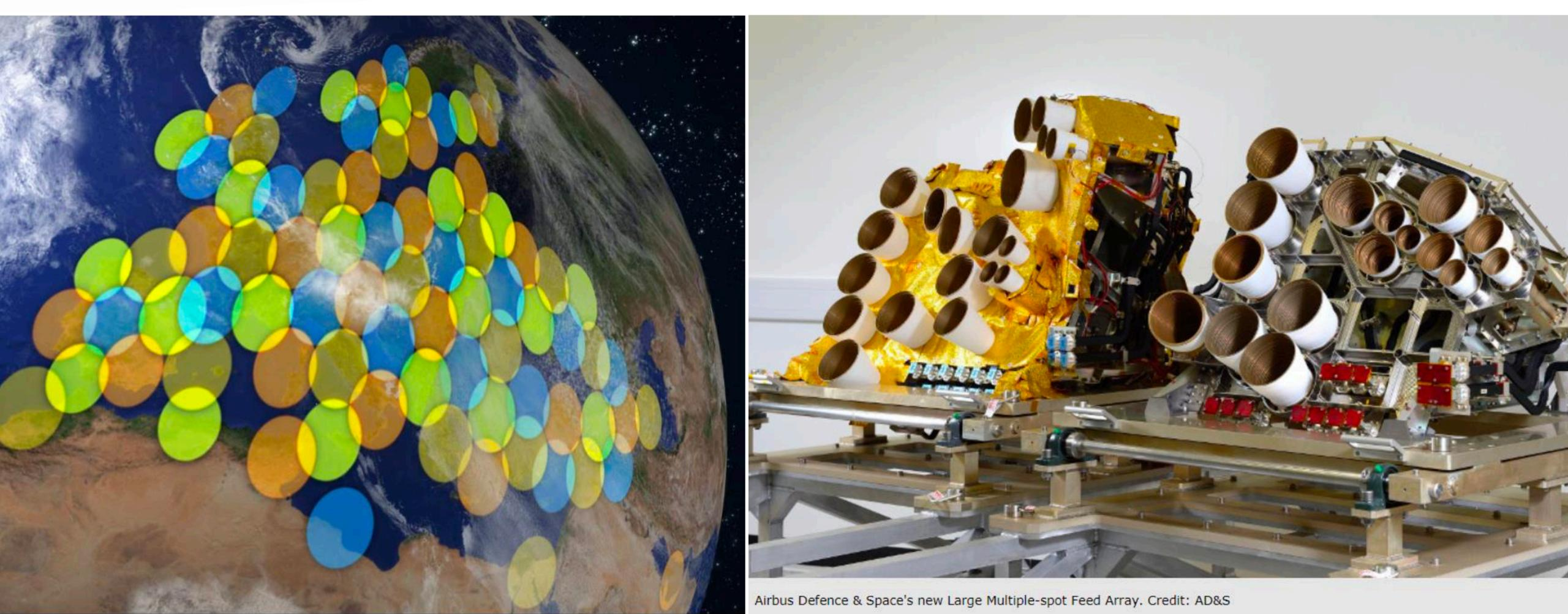
Spot beam antennas allow for spectrum reuse
