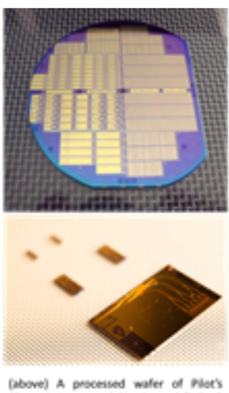
Photonic Integrated Circuits and (below) individual PICs after coating & dicing
