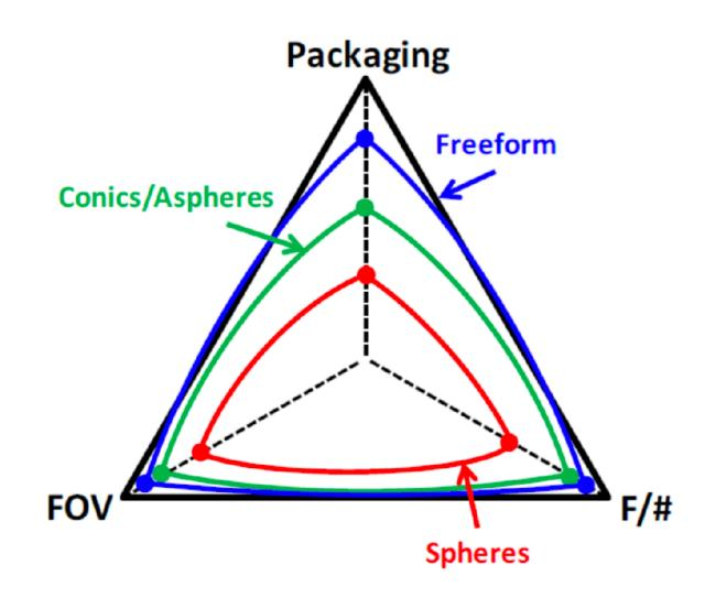
Image source: K. Fuerschbach. Freeform, φ-polynomial optical surfaces: optical design, fabrication and assembly. PhD thesis, Institute of Optics, Rochester, 2014
