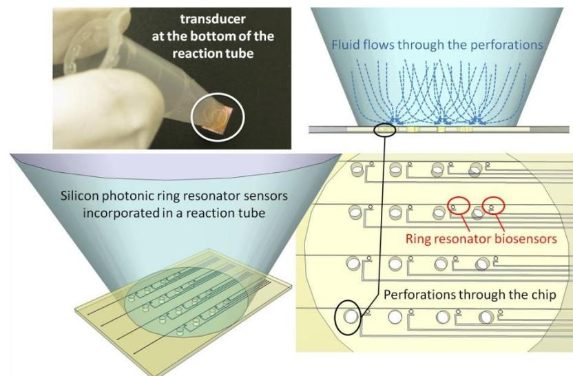
The silicon-on-insulator chip with the photonic biosensors and the embedded micro-fluidic system is incorporated at the bottom of a reaction tube.
