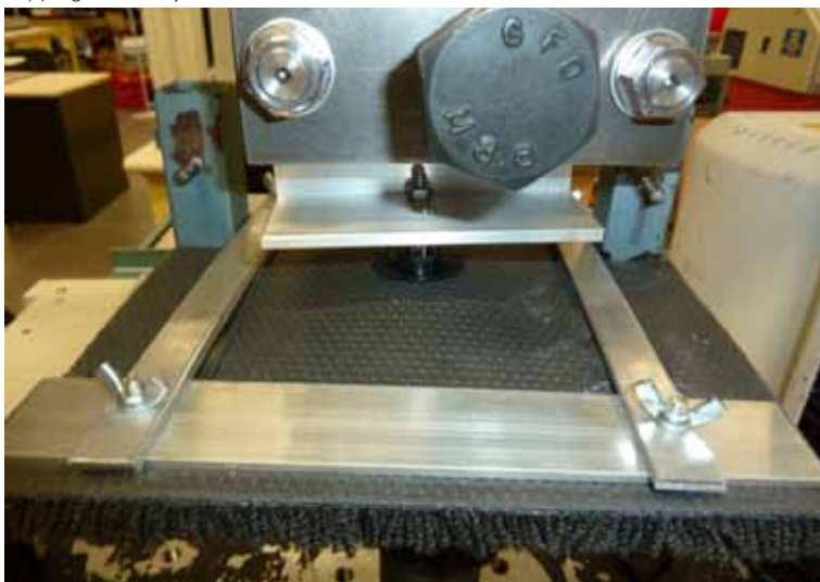
Flammability test for floorcoverings
