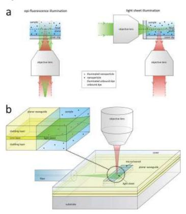
Microfluidic chip with integrated waveguide for light sheet illumination
