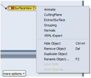
To extract a surface file now, right click on the white triangle in the **SurfaceView** module, which opens a drop down list. Then select **ExtractSurface**, after which the (red) module appears in the network. Click 'Apply' in the Properties window, and a separate surface module is generated for that material selected. To save that, click the **ExtractedSurface** module, and go to 'File' and 'Save As'. There select the file format needed.
