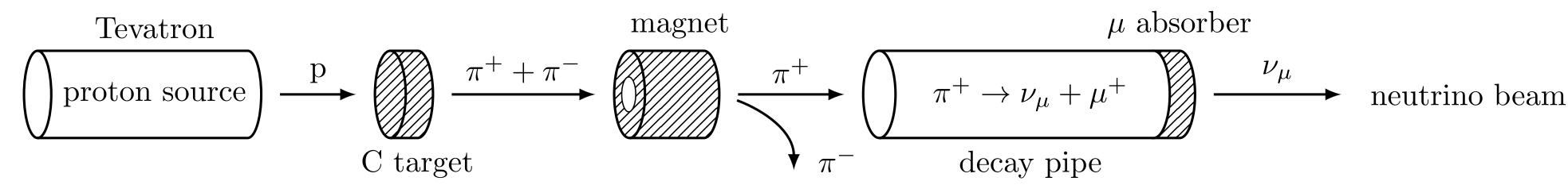
Colliding high energy protons (p) into a carbon target produces pions  $(\pi)$ , which are subsequently separated according to their electrical charge using a magnet. These pions then decay, creating neutrinos ( $\nu$ ) and muons ( $\mu$ ). The latter are filtered out.
