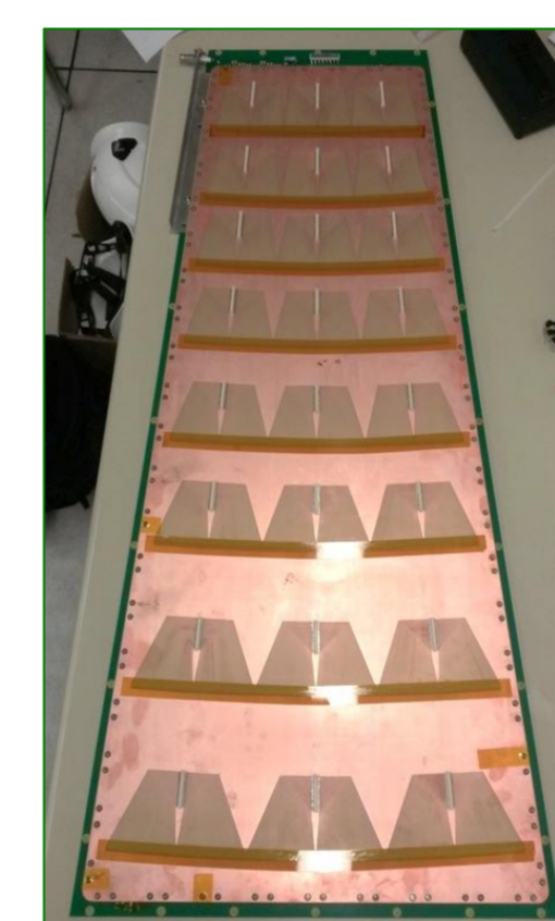
GE1/1 prototype after mounting the readout board onto the GEM foil stack
