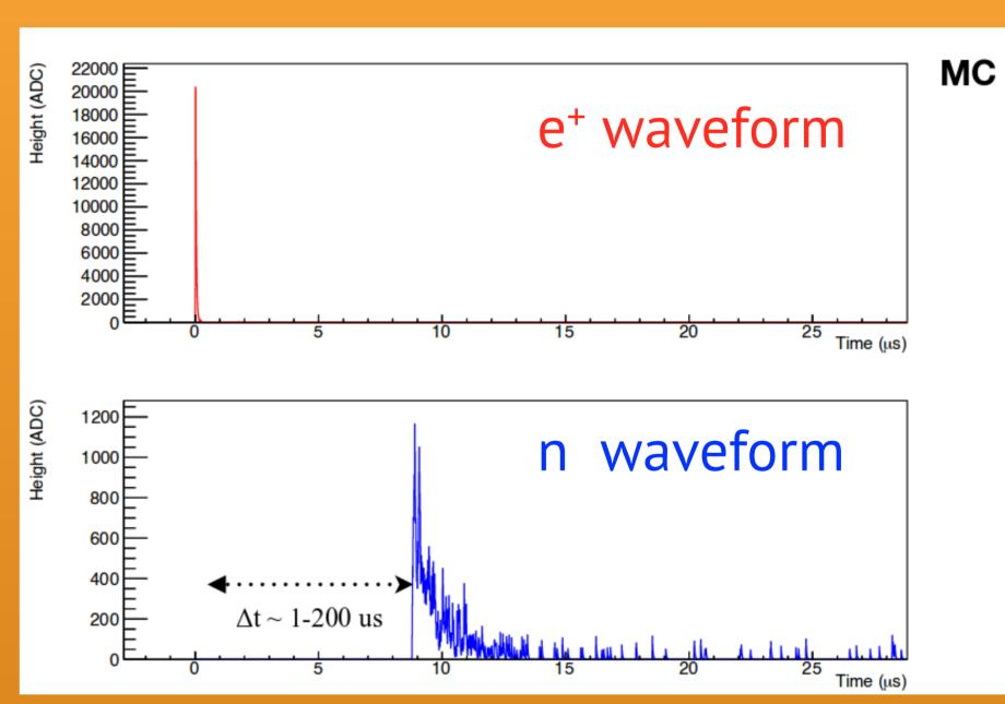
Pulse shape discrimination to identify the particles
