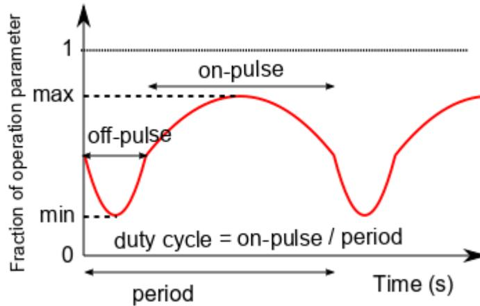
Definition of sinusoidal pulsing of operation parameters.
