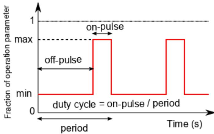
Definition of block pulsing of operation parameters.
