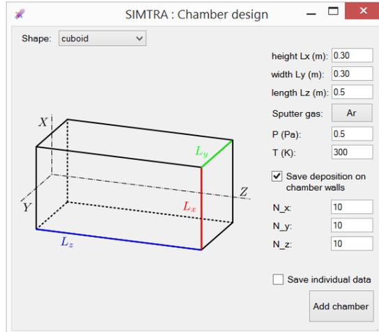
Figure 1: The Chamber Design window.
