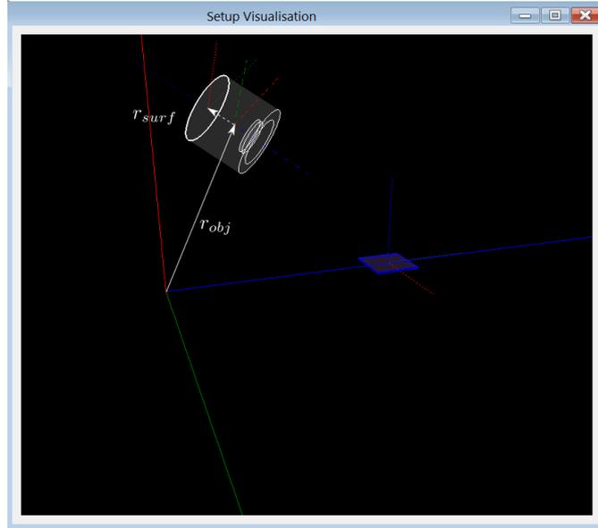
Figure 9: Illustration of the different reference frames: the position of the object  $r_{obj}$  is defined in the global reference frame. The position of the circular backside of the magnetron  $r_{surf}$  is defined in the reference frame of the magnetron (dashed lines).
