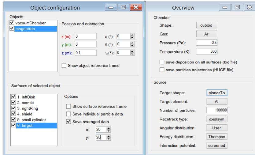
Figure 4: The Object Configuration and Overview windows.
