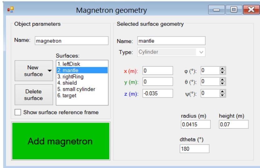
Figure 2: The magnetron geometry window listing the six surfaces of a predefined planar magnetron.
