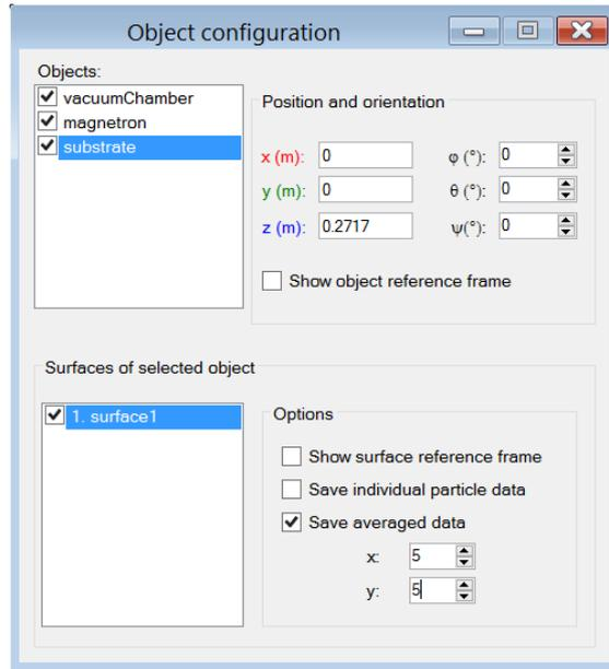
Figure 6: Defining a rectangular substrate of  $5 \times 5\text{ cm}^2$ .
