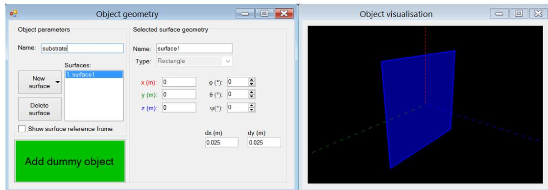
Figure 5: Defining a rectangular substrate of  $5 \times 5 \text{ cm}^2$ .
