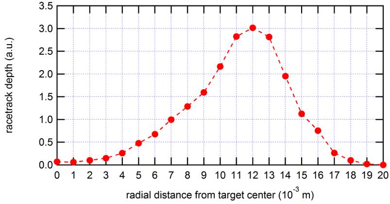
Figure 13: Example of a racetrack file in case of an axial symmetric racetrack.
