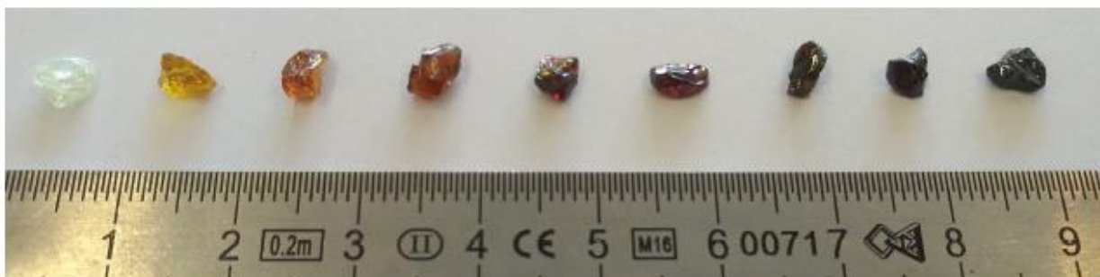
Figure 1 : Lead silicate glasses with a \text{PbO}/\text{Fe}_2\text{O}_3 weight ratio of 70/30 and increasing \text{Fe}^{3+} concentration (0 – 7 weight%), taken from [1].
